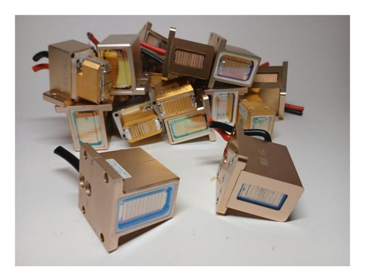
Diode emitter 808 nm for the handle of the epilator
