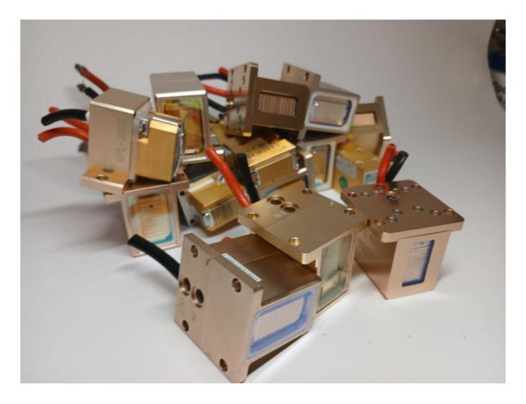
Laser radiation block for the handle of a cosmetology device
