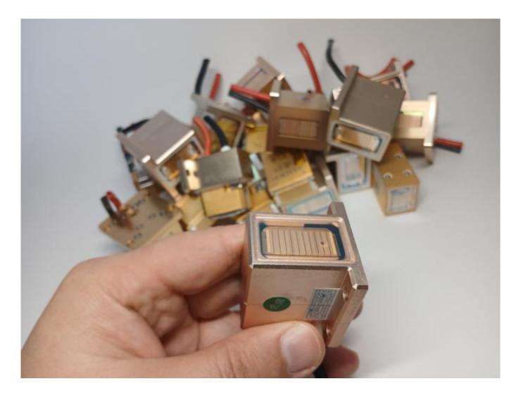
Replacing a diode stack in the handle of a cosmetology device
