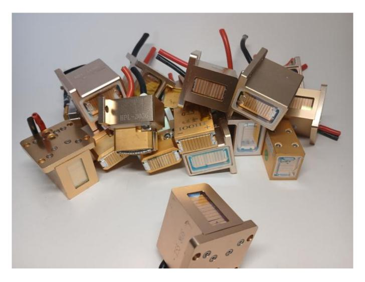
Laser stack for a diode laser manipula
