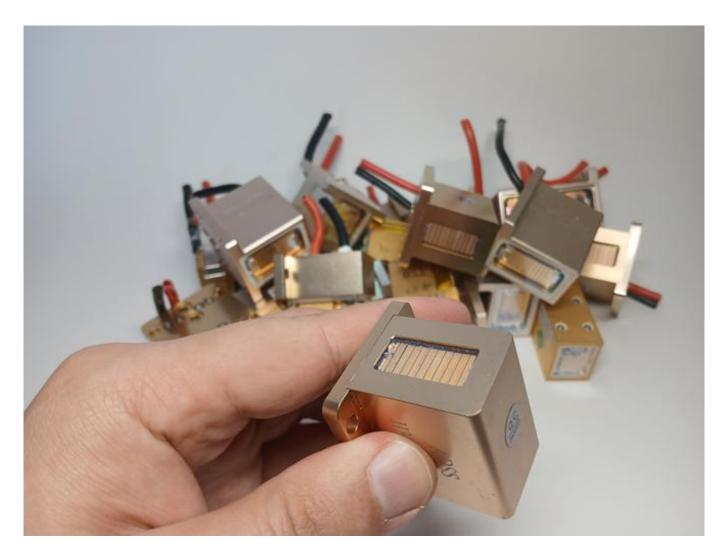
Diode emitter for the handle of the laser apparatus
