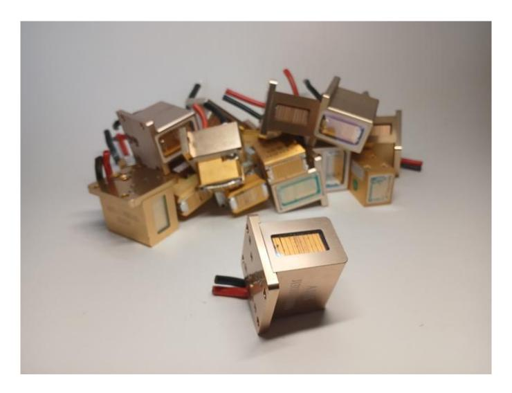
Laser diode module for the handle of the epilator
