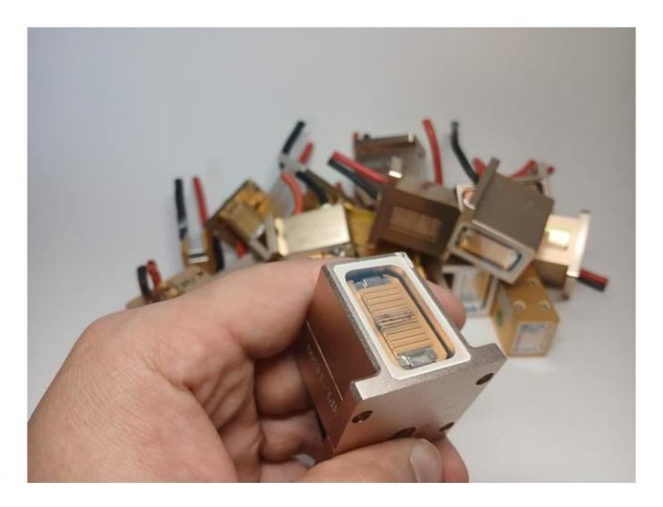
Replacing the laser cluster in the handle.
