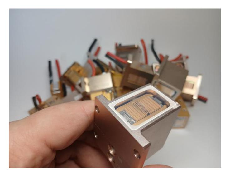
Repair of a manipula with a complete replacement of the laser.
