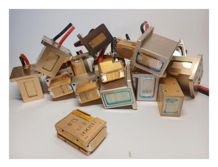
Repair of a laser head with a replacement of diodes.
