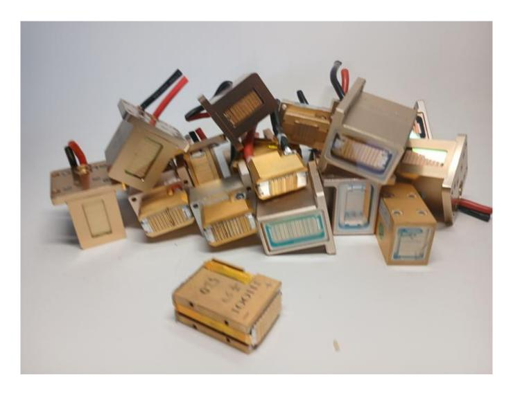
Restoring the laser function of the manipula by replacing diodes.
