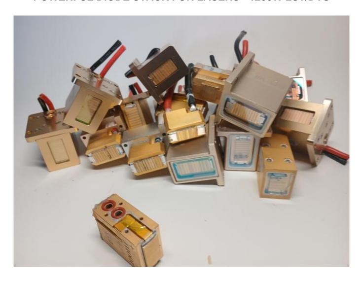
Service replacement of a diode stack.
