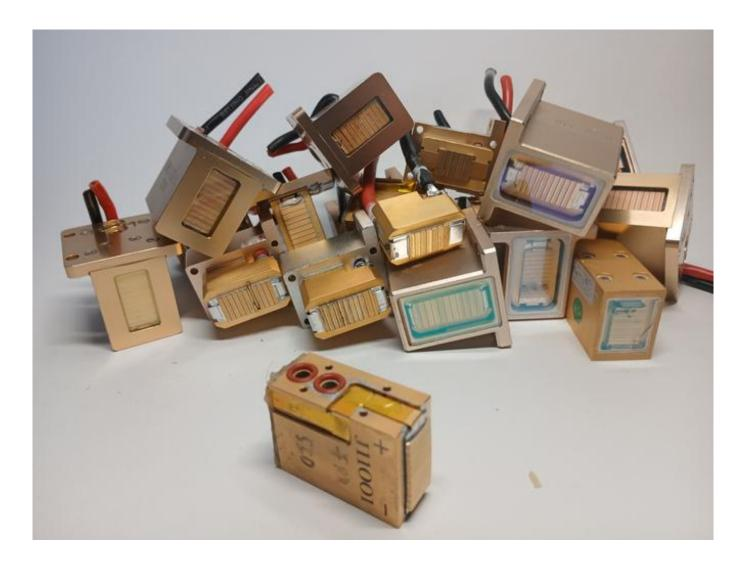
Non -working handle of a diode laser
