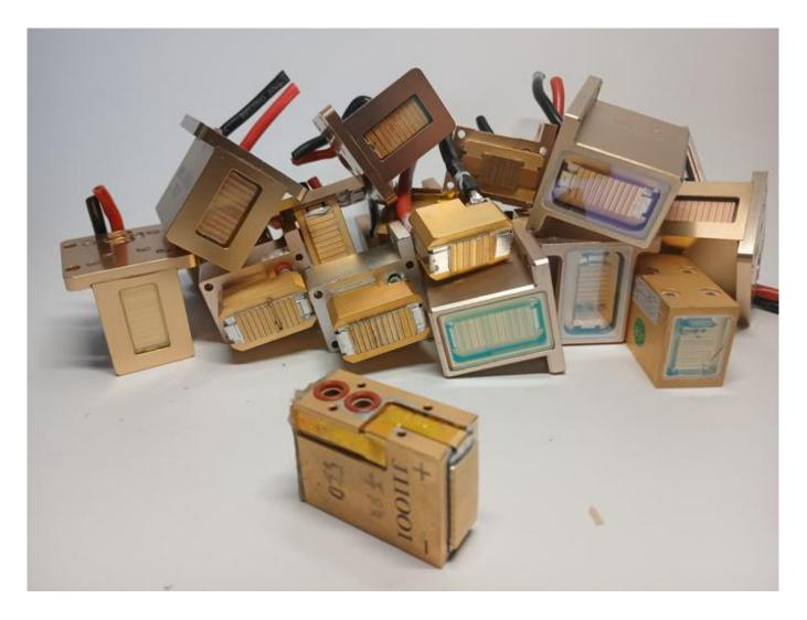
Restoring the manipula by changing the diode module.
