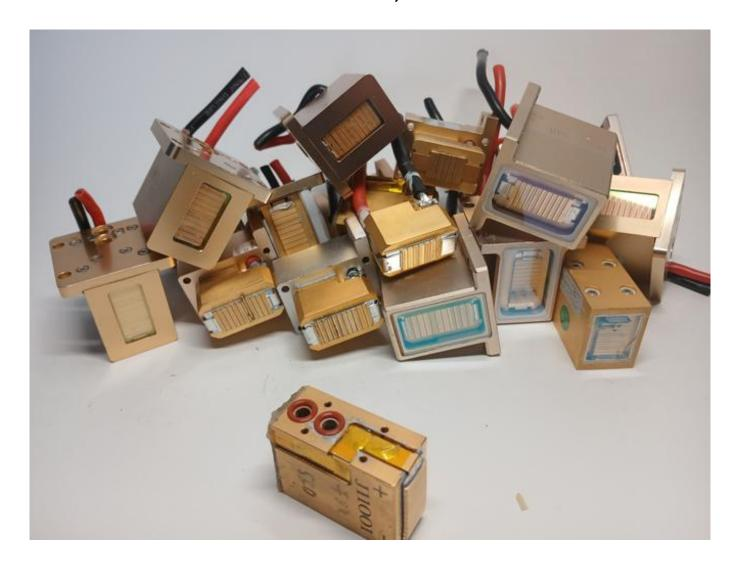
Complete replacement of the laser radiation source in the handle.
