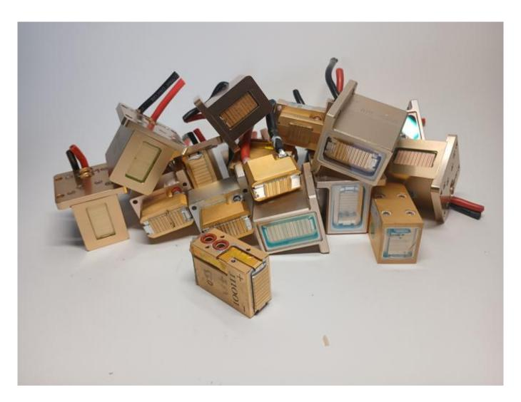
Repair and repaired diode stack in Laser.
