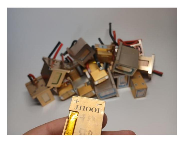
Repair of a diode stack in the laser handle.
