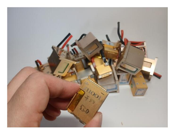
Maintenance: replacing a diode stack in a handle.
