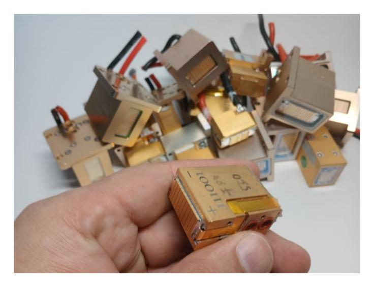
Change of diode board in the manipule of a cosmetological laser.
