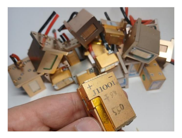
Service update of diodes in the handle of the apparatus.
