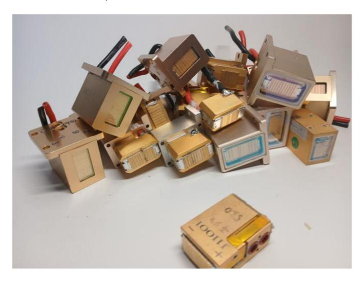
Replacing the diodes module in the laser handle.
