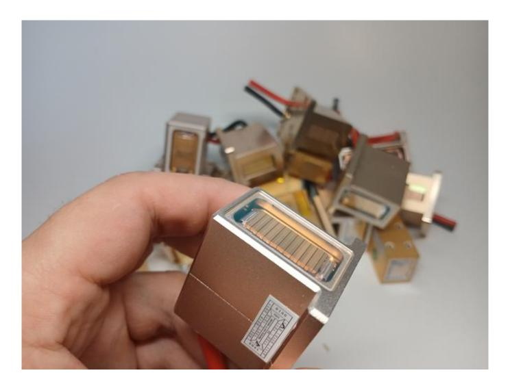
Restoring the manipula through the replacement of the module.
