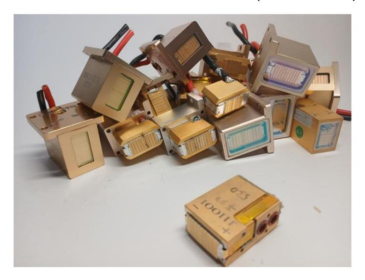
What is the diodes module in the laser?
