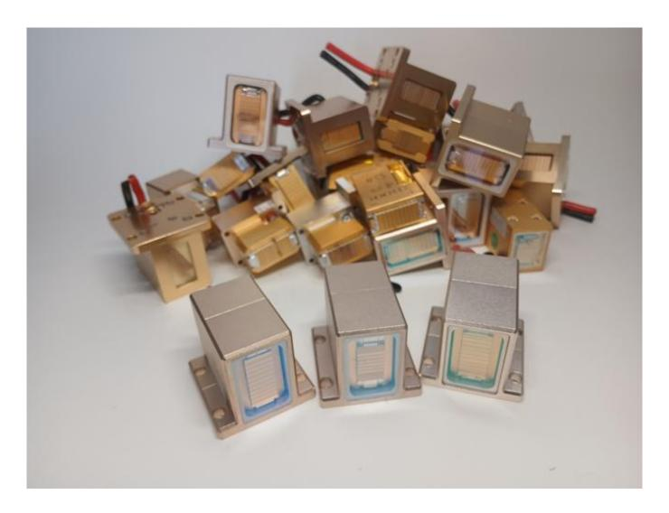
Complete replacement of the laser block in the manipul.
