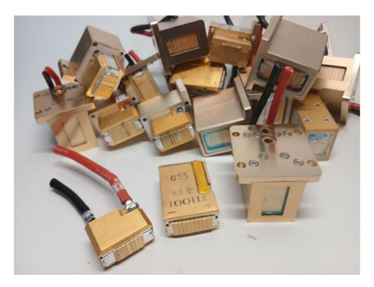
Replacing the failed diodes in the handle.
