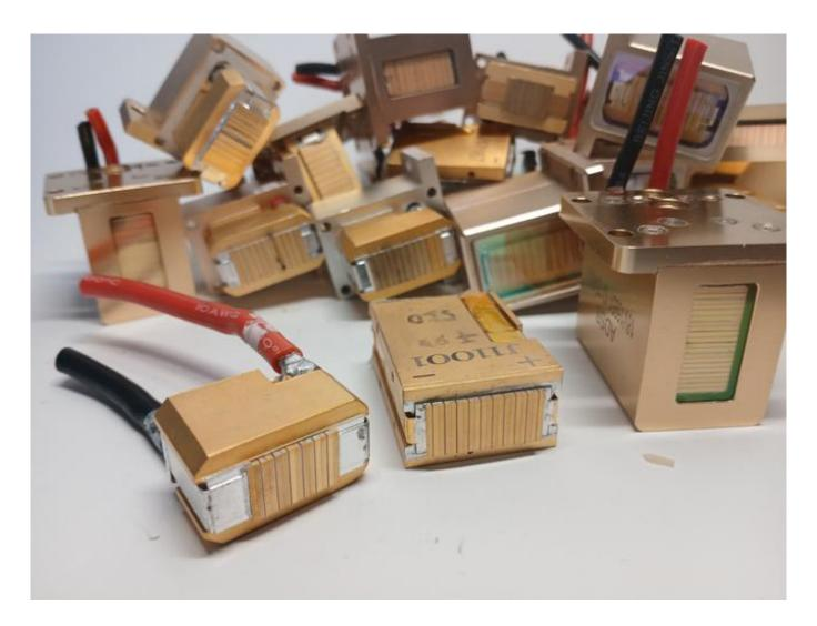
Restoring the power of the laser through the replacement of diodes.
