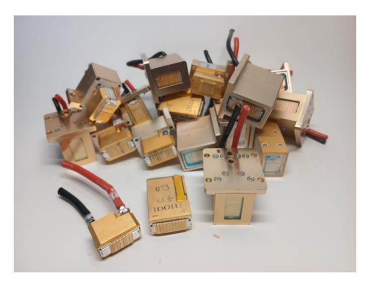
Change of the internal module of the laser handle.
