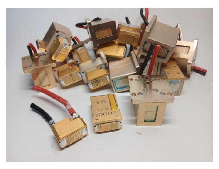
Full dismantling and installing a new diode stack.
