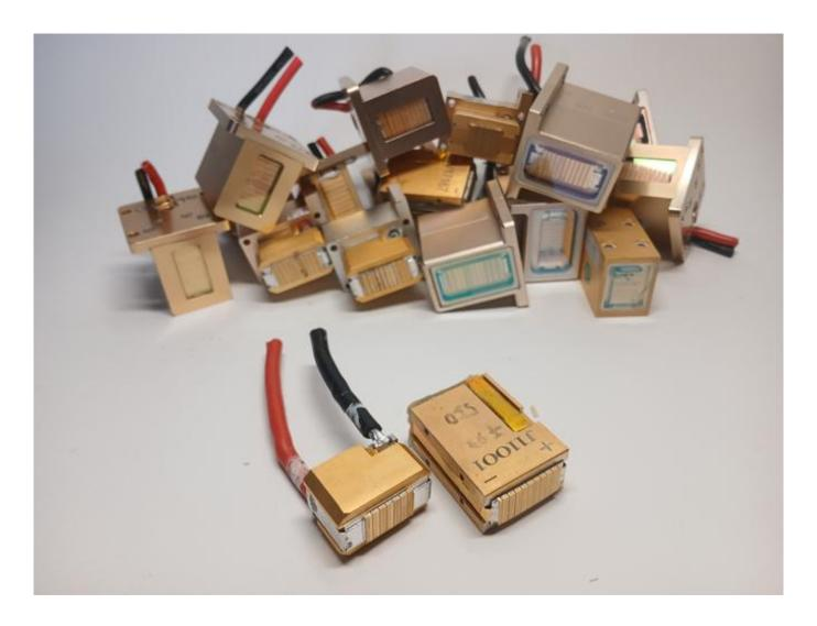
Laser handle maintenance with a complete replacement of diodes.
