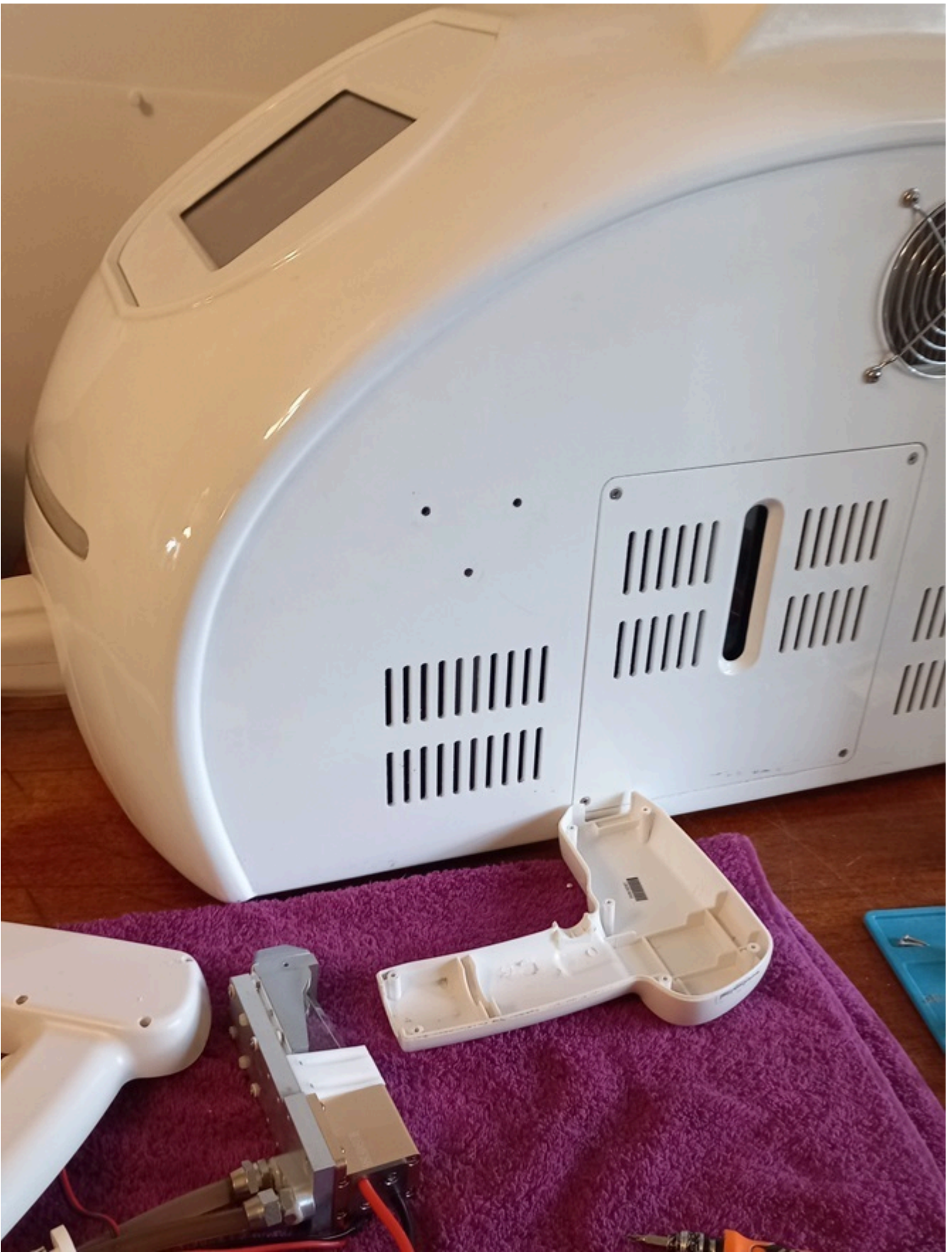
The photo shows the already replaced laser module of the ADSS diode laser handle.
