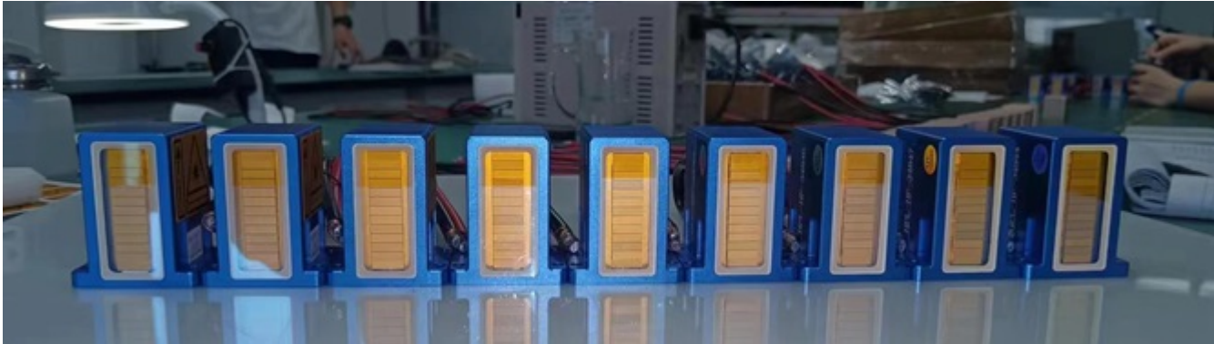
Diode array 1200 watt 12 bar 808nm, 1000 watt 10 bar 808nm, 800 watt 8 bar 808nm.
