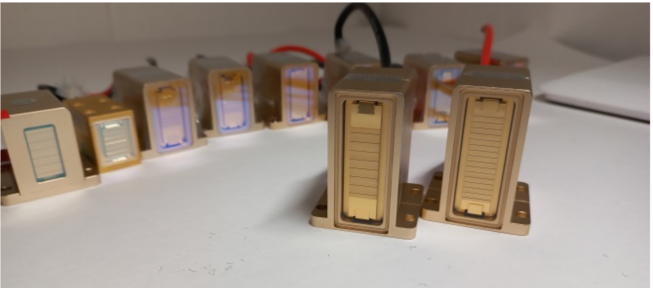
The photo below shows a 500 watt 10 bar and 600 watt 12 bar diode stack for Alma copy diode laser pens. This stack is 49 mm high, versus the standard 37 mm high.
