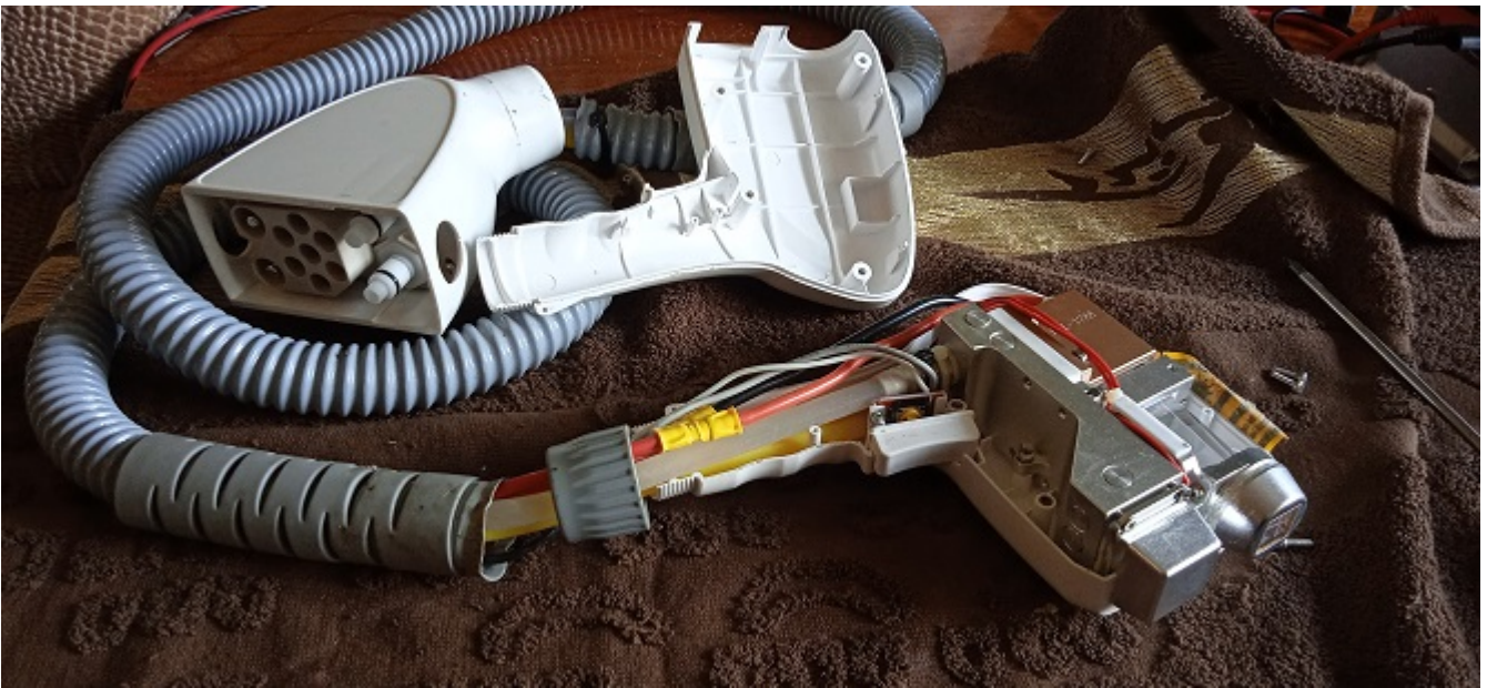
This laser pen came from one region of Russia. There was a complaint that there were no flashes when the device was turned on.
