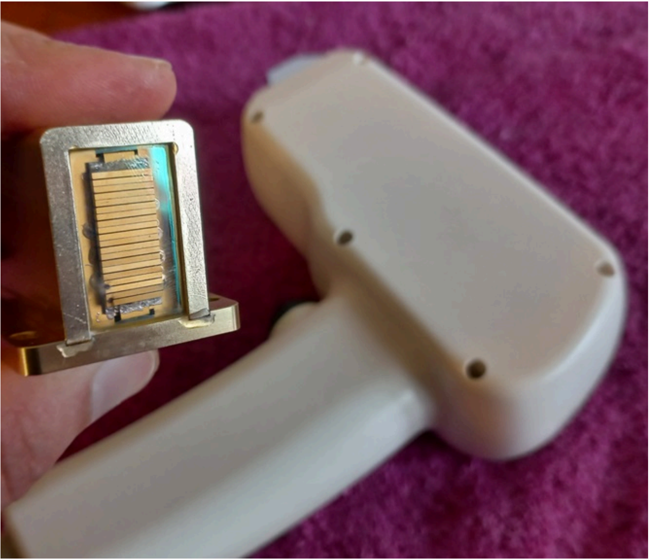
This is what a 500 watt 10 bar stack looks like, which was replaced with a new one.
