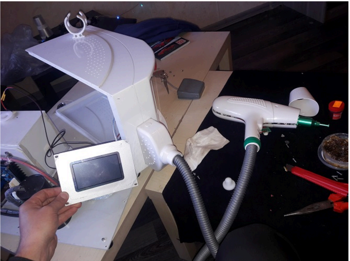
As for Chinese neodymium lasers, connectors often fly out during transportation... unless of course they are glued on))
