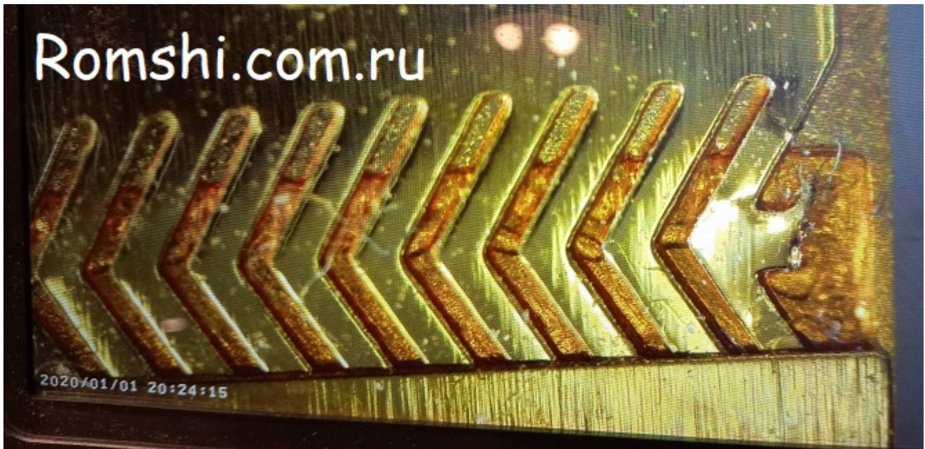
This photo shows slight wear of the micro channel plate from the stack.
