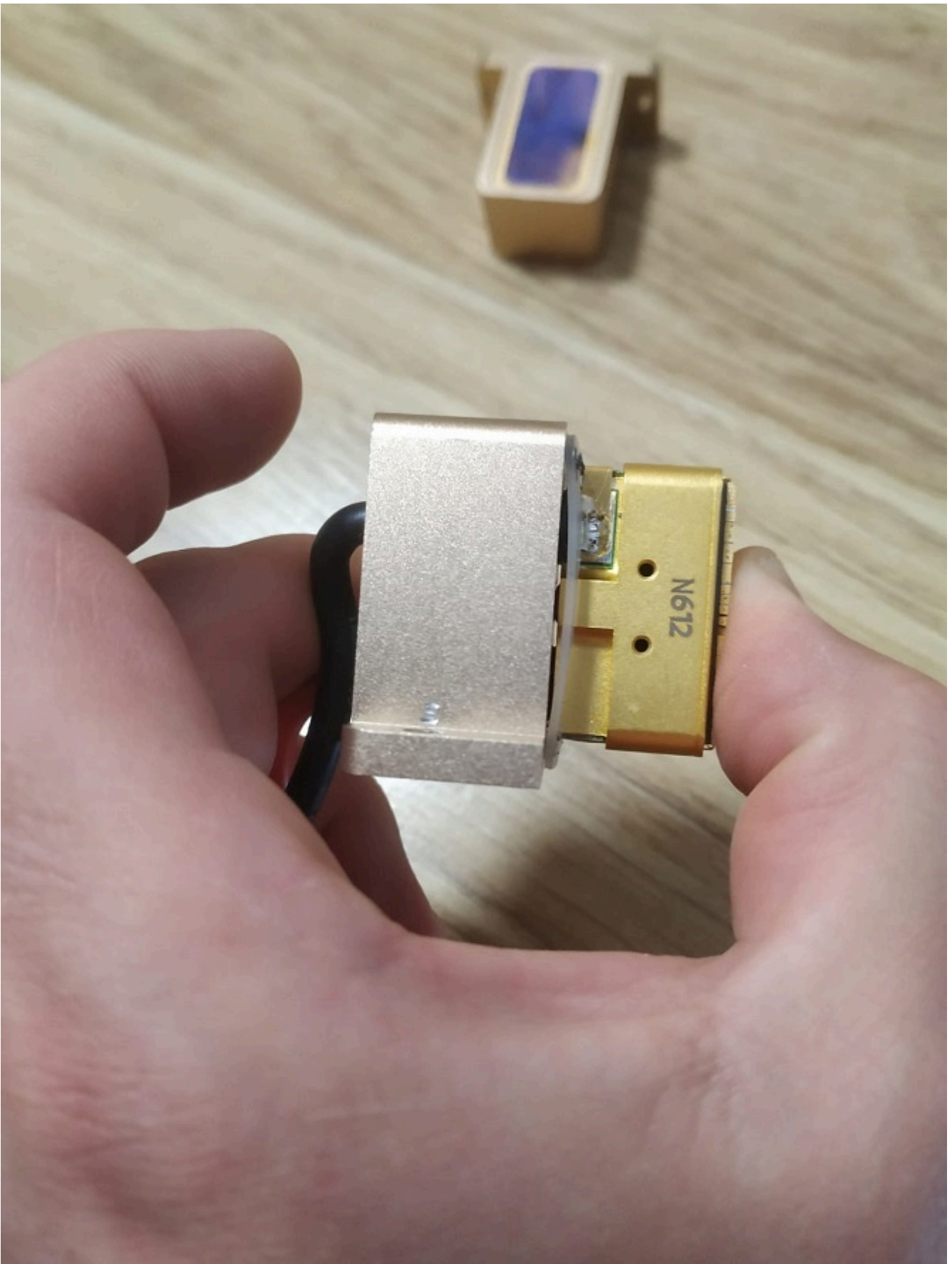
This stack was installed in this Chinese-made laser diode.
