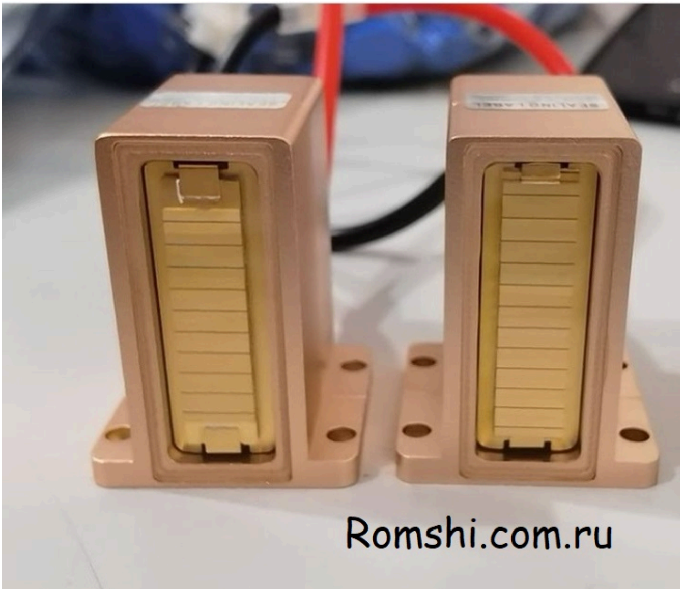
The photo below shows an example of an ozero khanka ok 01 laser handle. This diode stack handle contains a 300 watt 6 bar laser emitter.
