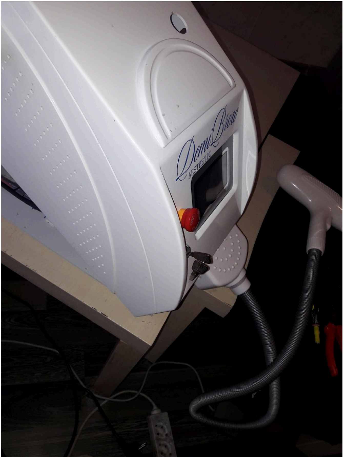
The Nd:YAG laser pen contains water cooling and wires that power the lamp. In this case there was also a pilot beam.
